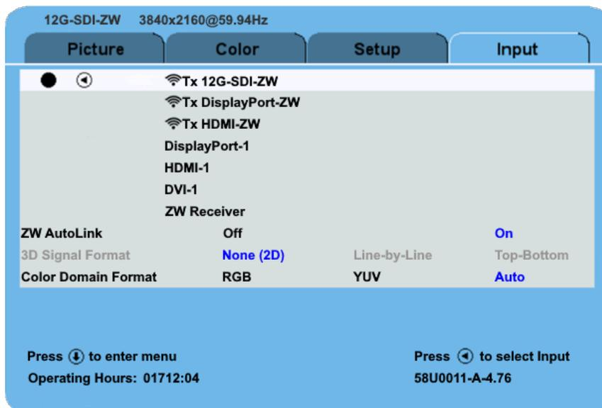
Open the Input Menu directly by tapping the **INPUT** button.
